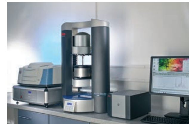
Modular rheometer platform HAAKE MARS with Rheonaut module and Thermo Scientific™ Nicolet™ iS10 FT-IR spectrometer
