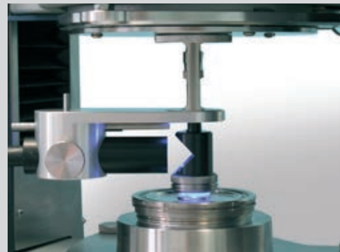
UV curing cell
