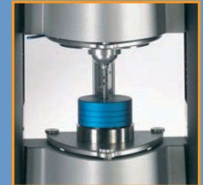
Temperature module for parallel plates with insulated sample hood
