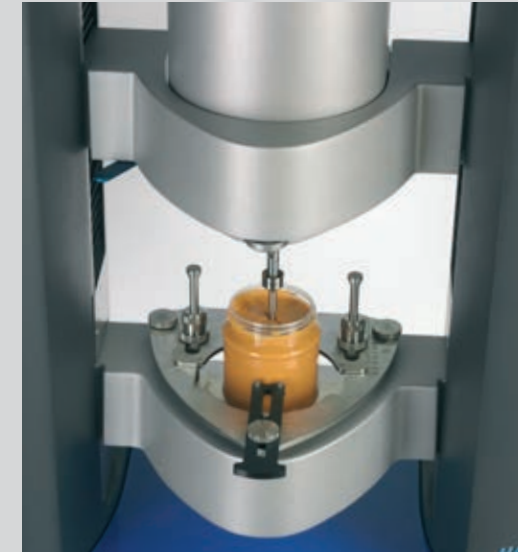
Peanut butter measured with HAAKE MARS, universal container holder and vane rotor
